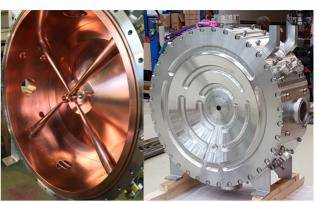
Figure 4: Photo of CH cavity 1 after copper plating (left) and ready for high power tests (right).
