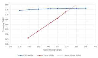
Figure 3: Measured tuner sweep of CH cavity 1 with expected tuner mode in tuning range. The Tuner position is measured from the DN100 CF flange.
