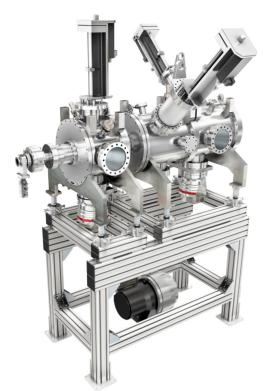
Figure 5: Setup of the Diagnostic Bench. Components on beam axis from left to right: Gate valve, ACCT, BPM, SEM, Emittance meter, BPM (hidden).
