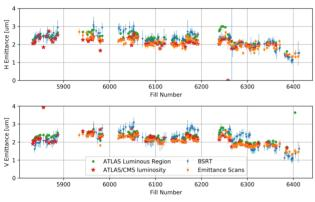
Figure 1: Emittances estimated using different instrumentation techniques at the start of collisions.
