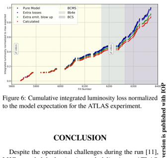
Figure 6: Cumulative integrated luminosity loss normalized to the model expectation for the ATLAS experiment.
