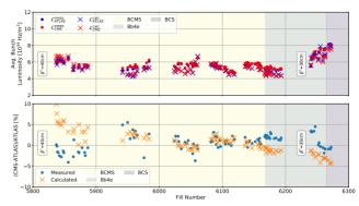
Figure 5: Comparison of the measured and calculated average bunch peak luminosity and the imbalance between the two high luminosity experiments.
