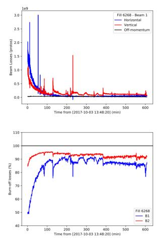
Figure 4: Evolution of the beam-1 losses for a selected fill, deconvolved for the two planes and the off-momentum protons, as seen by the collimation system (top). Time evolution of the percentage burn-off losses for the two beams (bottom).
