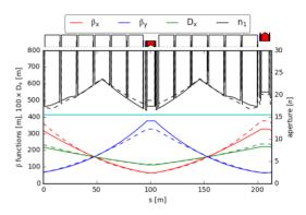
Figure 3: Optical functions ( $\beta_x$  in red,  $\beta_y$  in blue and  $D_x$ in green) in the FODO cell in the case of  $b_2 = 50$  (full line) and  $b_2 = -50$  (dashed line). The physical aperture in  $\sigma$  at injection energy of 3.3 TeV is shown in black. The target aperture of 15.5  $\sigma$  is plotted in cyan.
