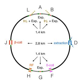
Figure 1: Layout of the FCC-hh ring.
