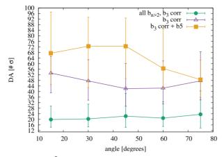
Figure 3:  $10^5$  turns dynamic aperture for 5 directions  $\phi = \arctan(\sqrt{\epsilon_y/\epsilon_x})$  of the space and 60 seeds. FCC injection optics without systematic  $b_2$  in the dipole and with nominal tunes 110.28/108.31. Dipole errors table v2.
