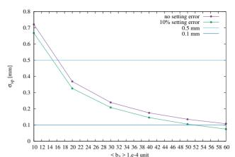
Figure 1: MCS random alignment to have  $\sigma_{b_2}^{\text{feed-down}} =$  $0.9 \cdot 10^{-4}$  as a function of the systematic  $b_3$  value at injection.
