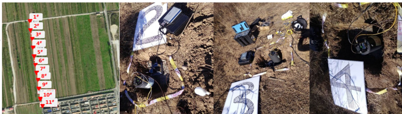
Figure 3: The positions of eleven pits distributed on HEPS site for ground motion measurement (left), the IHEP seismometers in the hole for the wave velocity measurement (middle and right graph).
