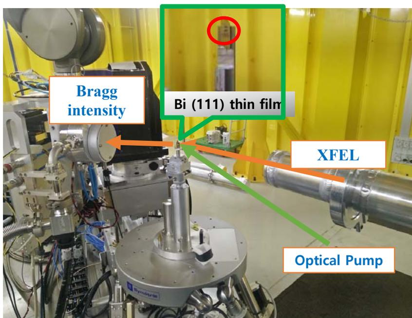
Bi(111) thin film (50 nm) on GaSb(111)/Si(111)
