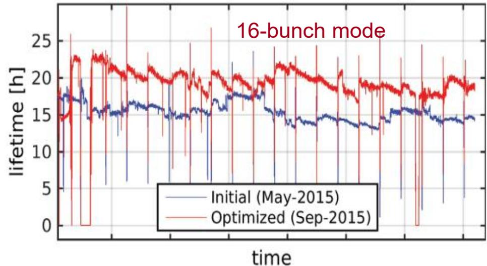
Multiple benefits: increased lifetime; using one lattice for both high and low bunch current modes; higher single bunch current, etc.
