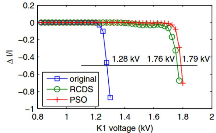
The kicker voltage is converted to kick angle and used in tracking to find out the dynamic aperture.
