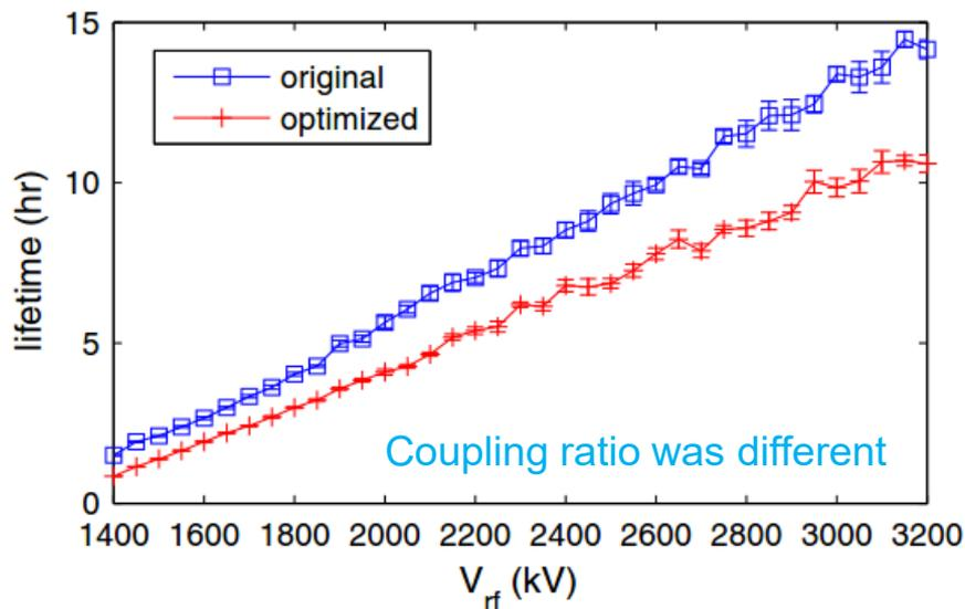
The difference in lifetime in the comparison is due to change of coupling ratio (vertical beam size).
