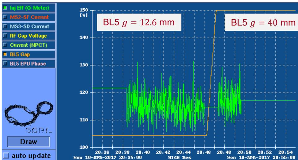
After optimization, injection efficiency is not impacted by BL5 gap changes.
