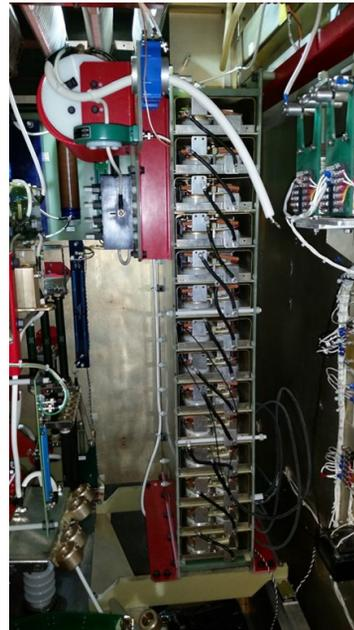
Figure 1: Final Power Amplifier High Voltage Switch Assembly. Switch consists of 14 IGBT switch plates and incorporates thick copper baseplates for inertial.
