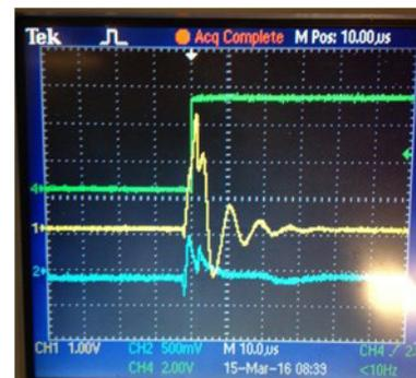
Figure 3: Full voltage Wire Test at Alcatraz C-Mod. Waveform shows data from the FPA at 31.4kV. Green: Fault Detection. Yellow: Switch Current. Once current threshold of 170 A is crossed, fault logic toggles to high and opens the switch. The current reaches 320 A before the switch opens.
