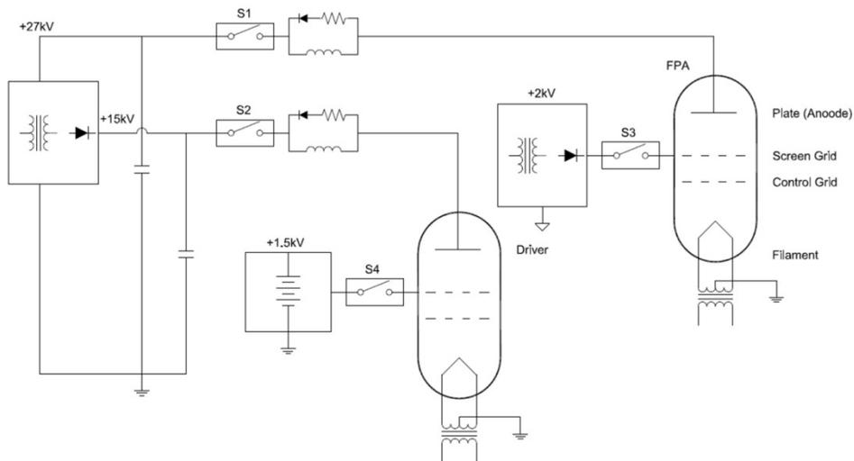
Figure 2: High Voltage Upgrade Schematic.
