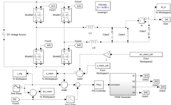
Figure 4: TPS quadruple magnet power model.
