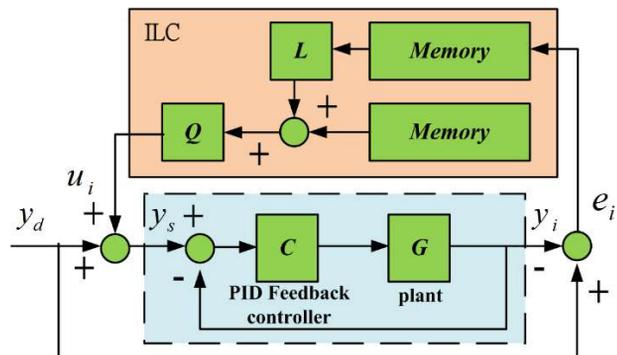
Figure 2: ILC feed forward with PID feedback control.
