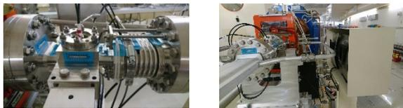
Figure 1: Monitoring location for the PT100 and thermal labels (left). Fan cooling system (right).
