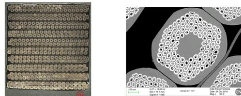
Figure 1: Cross section and micrograph of a Nb<sub>3</sub>Sn Cable.
