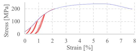
Figure 6: Compression tests over MQXF Samples.
