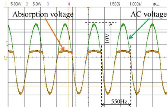
Figure 6: Measurement result of the terminal voltage when the absorption circuit SiC-MOSFET was turned off.
