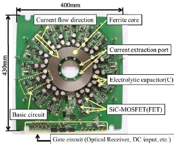
Figure 2: Picture of the new main LTD modules.
