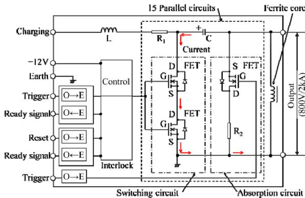
Figure 1: Basic circuit of the new main LTD module.
