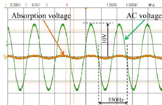
Figure 7: Measurement result of the terminal voltage when the absorption circuit SiC-MOSFET was turned on.
