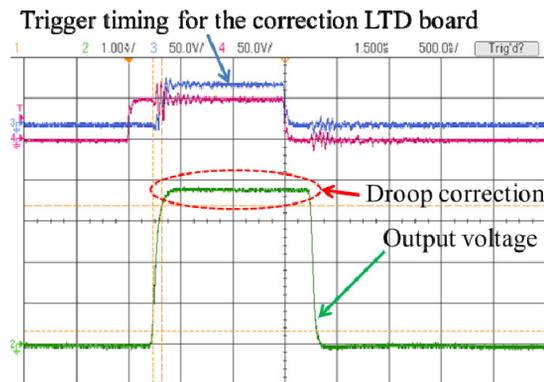
Figure 5: Measurement result of the prototype power supply when the flat top corrections were active.
