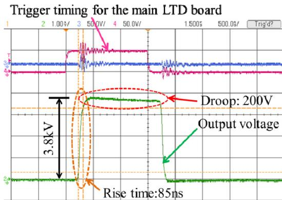
Figure 4: Measurement result of the prototype power supply when only the main circuits were operated.
