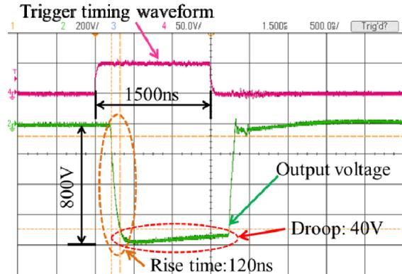
Figure 3: Measurement result of the output voltage waveform at one main LTD module.
