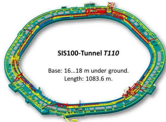
Figure 1: Overview of the lowest underground level of T110.
