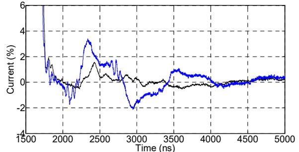
Figure 8: Measured PPR (current) before (blue) and after (black) the EYETS upgrade.
