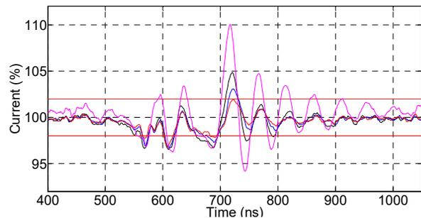
Figure 4: Measured current at the output of module 4 for different coils with two (black), three (blue) and four (red) turns mounted to the SC-plug and a direct SC (magenta).
