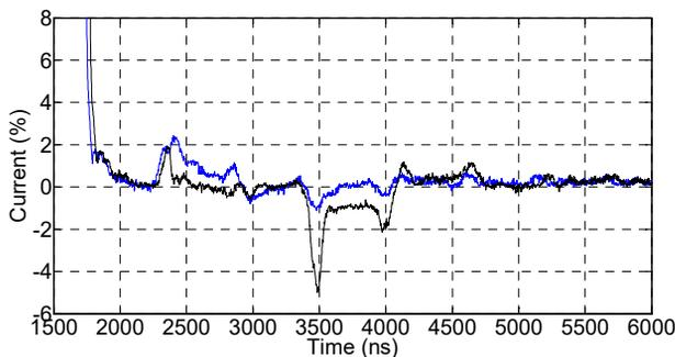
Figure 3: Measured post pulse ripple current of module 1 with five (blue) and three (black) LEMO ferrites.
