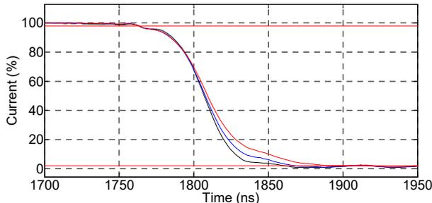
Figure 6: Current fall time measured at the output of module 4 for different coils with two (black), three (blue) and four (red) turns mounted to the SC-plug.
