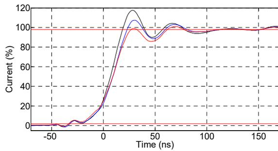
Figure 5: Current rise time measured at the output of module 4 for different coils with two (black), three (blue) and four (red) turns mounted to the SC-plug.
