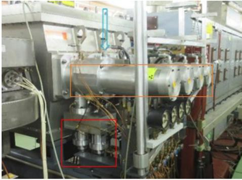
Figure 2: KFA-45 magnet after EYETS modifications: new magnet connection box extension (red), removed SC-thyratron and SC-plug (blue arrow) and TMR (orange).
