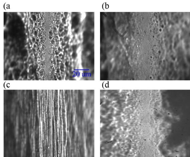
Figure 4: Images of the target rear surface. (a). 1.2  $\mu\text{m}$  thick aluminium target, (b). 2.5  $\mu\text{m}$  thick aluminium target, (c). 3  $\mu\text{m}$  thick titanium target, (d). 50 nm thick diamond-like carbon target, respectively. The scales of the figures are the same.
