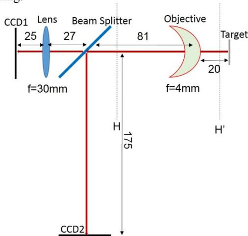
Figure 2: Schematic of the microscope system. The omitted unit is millimetre. Two different magnifications 10-fold (CCD1) and 50-fold (CCD2) can be achieved simultaneously with the help of a beam splitter.
