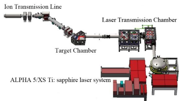
Figure 1: Layout of the CLAPA laser proton acceleration system.
