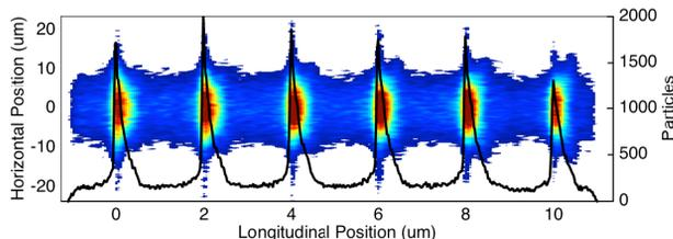
Figure 3:  $z-x$  phase space of a longitudinal 6 period slice of the simulated beam at the DLA entrance showing 6 consecutive microbunches. The black line corresponds to the projection across the horizontal axis (y axis on the right). Microbunch length:  $(699 \pm 88)$  as FWHM, spacing:  $(2.00 \pm 0.01) \mu\text{m}$ .
