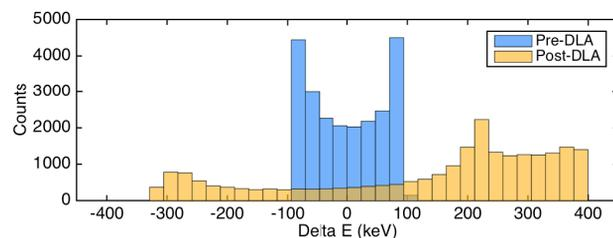
Figure 5: Simulated energy spectrum of the transmitted/collimated part of a 6 period slice of the modulated beam before and after the DLA interaction ( $\Delta E$  w.r.t the initial mean energy).
