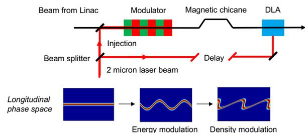
Figure 1: Basic representation of the microbunching scheme using a modulator and a chicane.
