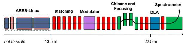
Figure 2: Schematic overview of the proposed beamline. The beam direction is from left to right. The schematic is not to scale. Red elements correspond to quadrupoles, green elements to dipoles.
