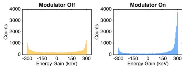
Figure 4: Simulated energy gain spectrum of the transmitted/collimated part of a 6 period slice after the DLA interaction. Acceleration is enhanced in the modulated case.
