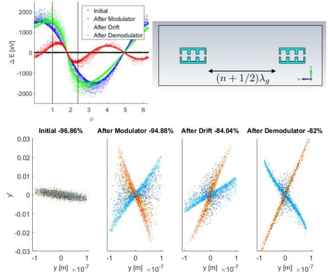
Figure 8: Longitudinal phase space and grating setup (top) and transverse phase space ( $y' = \gamma \beta_y$ ), where the color indicates the particle phase  $\varphi$  (bottom).
