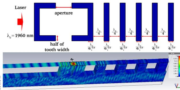
Figure 1: Bragg mirror cavity structure (Silicon  $\epsilon_r = 11.63$ , length  $\lambda_g = 620\text{nm}$ ) for  $n=0$  (top) and 3D simulation for  $n=3$  and height  $3\mu\text{m}$  (bottom). The black arrow indicates the electron trajectory at which the structure is periodic.
