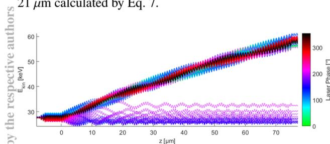
Figure 7: Energy gain along the structure for 72 particles launched at  $t = 0$  sweeping over the laser phase in steps of 5 degrees. The fraction of trapped particles is 81%.
