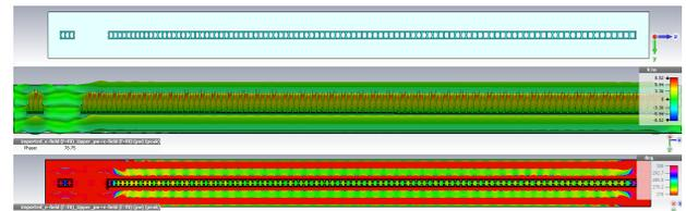
Figure 2: Chirped accelerator structure with 100 periods (top), longitudinal electric field amplitude (center), and phase (bottom) along the chirp.
