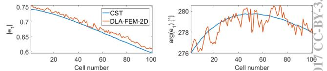
Figure 5: Establishing (almost) constant phase (4 deg jitter) by adjusting the tooth width.
