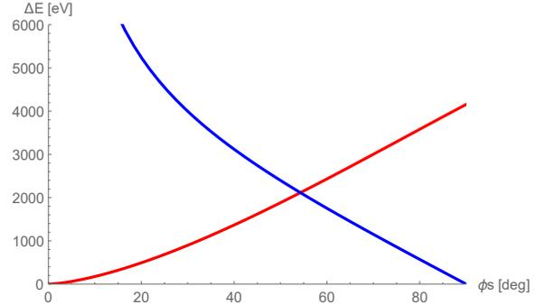
Figure 4: Energy spread acceptance (red) and energy gain per quarter synchrotron period (blue) as function of the synchronous phase  $\varphi_s$
