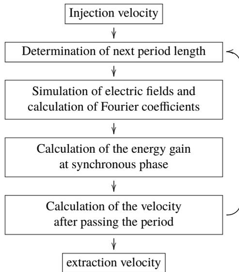
Figure 6: Iteration for the design of a chirped grating.
