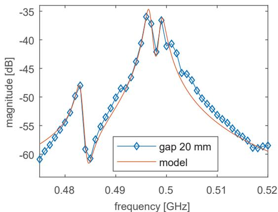
Figure 7: Measured  $S_{21}$  fitted over a small frequency range with a model of three second order resonators of  $f_0=483$  MHz, 496.56 MHz and 499 MHz with suitably chosen amplitudes and phases.
