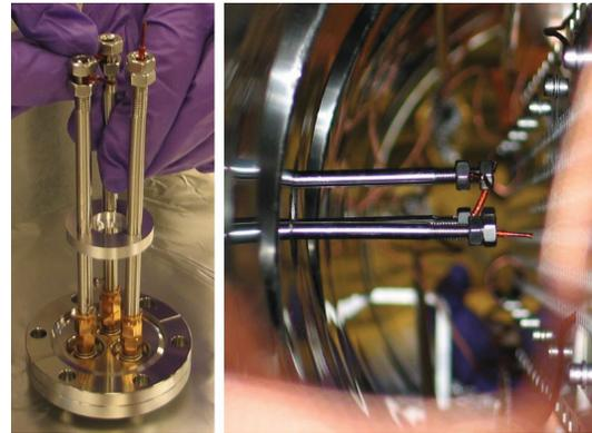
Figure 2: Left: View of the three in vacuum antennae during assembly. Right: View of the antennae installed in the ID, of which the shielding plates are visible on the right.
