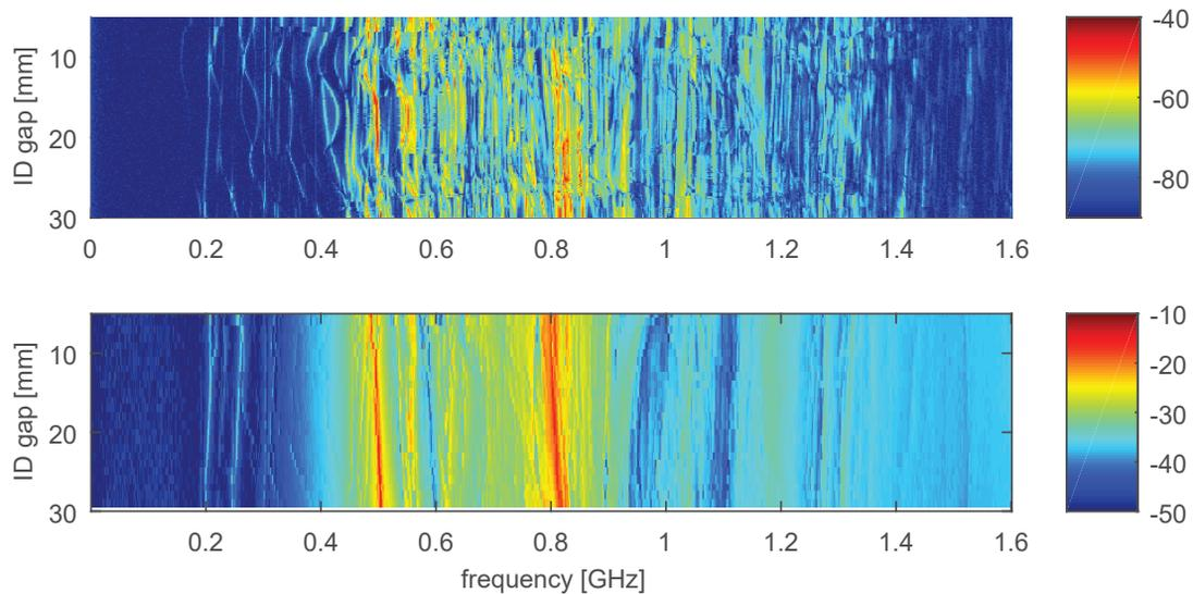
Figure 6: Comparison of single bunch spectra (colour-map in dBm) and  $S_{21}$  (colour-map in dB) over the same gap and frequency range.
