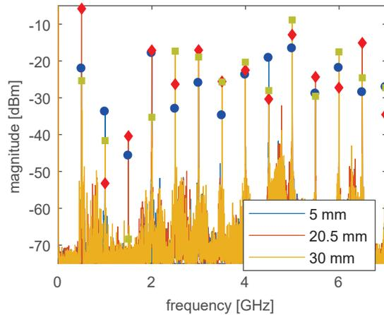
Figure 4: Spectra acquired from one of the antennae for 3 different ID gaps acquired with 300 mA stored beam in 900/936 bunches 'user mode'.
