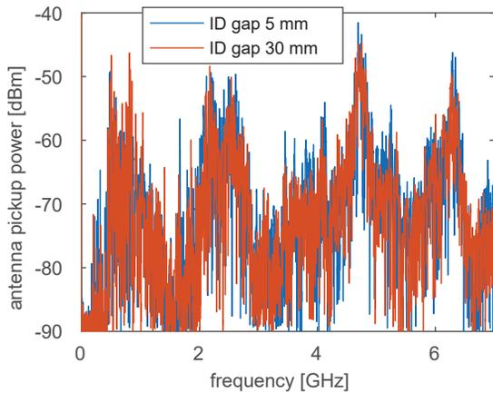
Figure 3: Spectra from one of the antennae for extremes of ID gap acquired with 2 mA single bunch stored beam.
