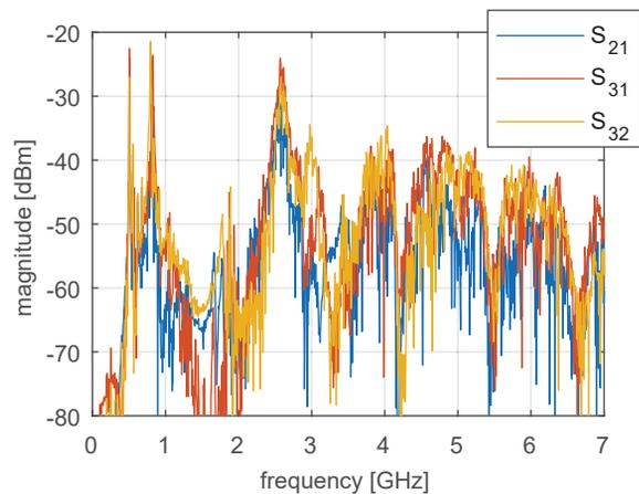
Figure 5: S-parameters acquired at the maximum ID gap with no stored beam.
