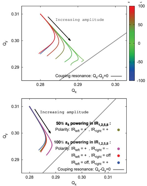
Figure 4: Detuning of particles towards the  $Q_x - Q_y$  resonance with increasing strength of  $a_4$  correctors in LHC insertions at injection (top). Detuning for various configurations of  $a_4$  circuits (bottom).  $|C^-| = 0.000$  in all cases.
