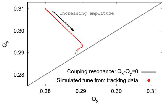
Figure 2: Detuning of particles towards the linear coupling resonance, with  $a_4$  errors and Landau octupoles included in the simulation.  $|C^-| = 0.000$  in this simulation.
