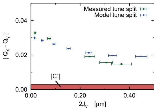
Figure 1: First observation of amplitude dependent closest tune approach [2].
