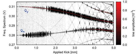
Figure 5: Frequency spectrum vs kick amplitude with 50 % powering in  $a_4$  correctors.
