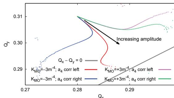
Figure 7: Approach to  $Q_x - Q_y = 0$ , for negative MO polarity with vertical kicks, and positive MO polarity with horizontal kicks. Only  $a_4$  correctors left of IR1 and 5, or only right of IR1 and 5, are powered.  $|C^-| = 0.0$  in all cases.
