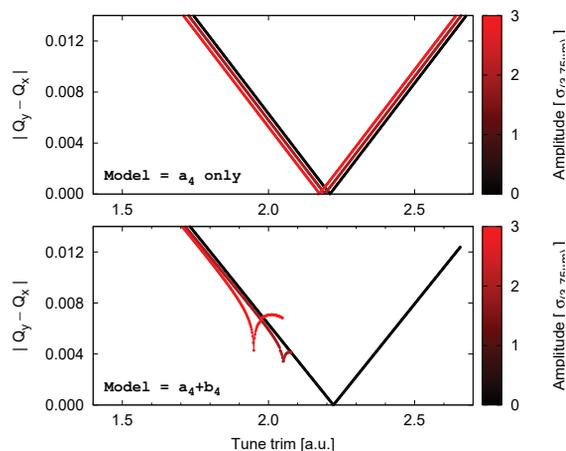
Figure 6: Tune separation in LHC models with only  $a_4$ , and with  $a_4$  plus  $b_4$  sources included.
