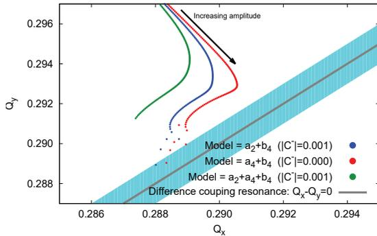
Figure 3: Approach to the  $Q_x - Q_y$  resonance for LHC simulations at injection, including various multipole sources.
