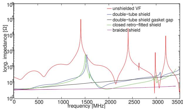
Figure 5: Comparison of simulation results for the longitudinal impedance of SPS vacuum flange connecting QF/MBA beam pipes for the unshielded case (red), vacuum flange equipped with double-tube shielding and gap filler (blue), and additional gasket gap closing (black), the retro-fitted shield (green) and the braided shield (violet). The closing of the gasket gap effectively suppresses the resonance seen at about 1.4 GHz/ 1.65 GHz.
