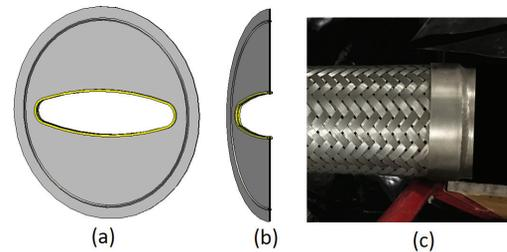
Figure 4: Re-designed gasket that closes the pill-box shaped gasket gap in front (a) and cross-sectional view (b). Woven wire structure of stainless steel for braided shield (c).
