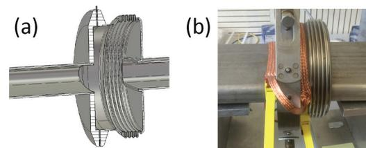
Figure 1: SPS vacuum flange. (a) Model of a QF/MBA flange without impedance shield, (b) Image of a QF/MBA flange installation in the SPS (with soft-clamp installed).
