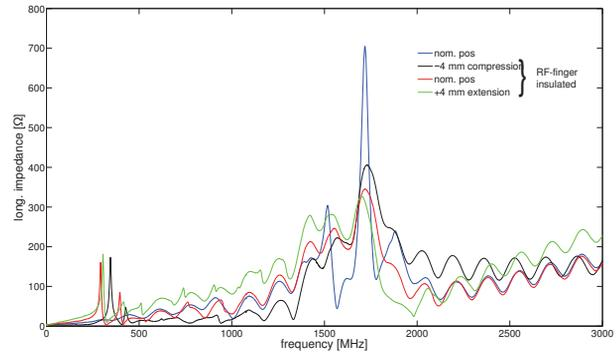
Figure 6: Wire measurement results of the retro-fitted shield prototype for nominal, extended (green) and compressed bellows (black) position as well as with (blue) and without insulated RF-fingers (red).
