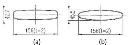
Figure 3: SPS vacuum chambers of the main bending magnet (MBA, (a)) and the quadrupole magnet (QF, (b)). Dimensions are shown in mm.
