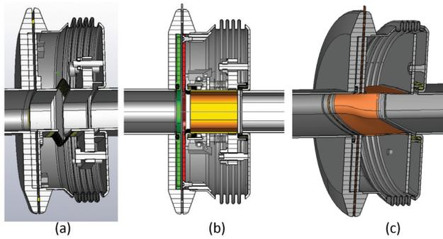
Figure 2: Vacuum flange with 4-convolution bellows for QF/MBA interface with double-tube shield (a), retro-fitted shield (b), braided shield (c).
