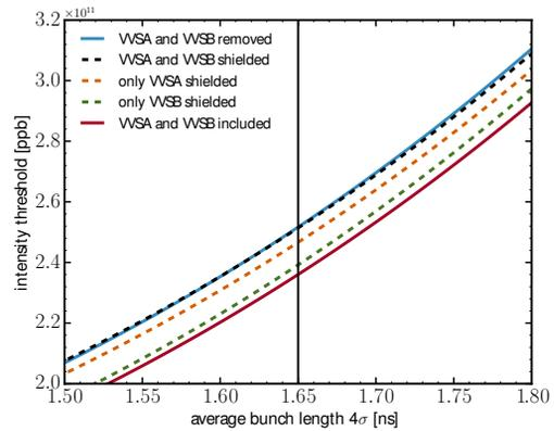
Figure 6: Results of macroparticle simulations (BlonD) for 72 bunches at SPS flat top in a double RF system (10 MV at 200 MHz and 1 MV at 800 MHz in bunch shortening mode) for the situation as expected after LS2. The plot shows intensity thresholds vs. average bunch length, for the situation with shielded and unshielded sector valves in the SPS ring. Three different scenarios for shielded valves are shown together with the case of no sector valves at all as well as the current status quo.
