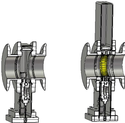
Figure 2: CAD model of a VVSA sector valve (left) and the impedance shielded version (right). The body of the shielded valve version is significantly larger than the unshielded one. The extended size is required for housing the impedance shield if the valve closes.
