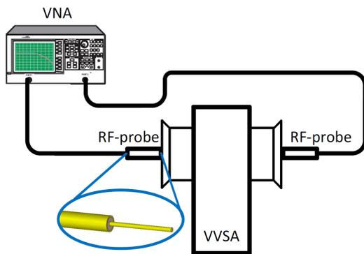
Figure 3: Schematic of the measurement set-up for benchmarking the EM-simulation model with S-parameter measurements via a vector network analyser (VNA). The inset shows the tip of the RF-probe.
