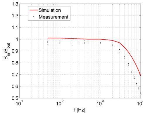
Figure 9: Amplitude attenuation versus frequency.
