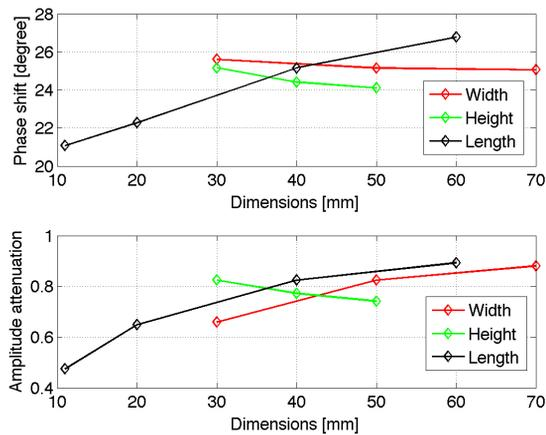
Figure 7: Dependence of phase shift (up plot) and amplitude attenuation (down plot) on the dimension of the coil.
