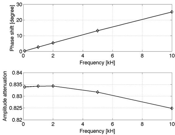
Figure 3: Dependence of phase shift (up plot) and amplitude attenuation (down plot) on frequency.
