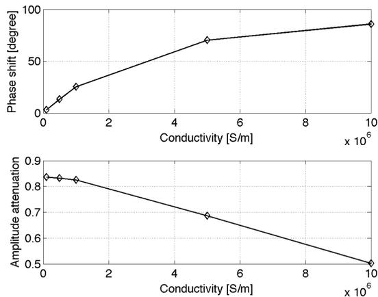
Figure 4: Dependence of phase shift (up plot) and amplitude attenuation (down plot) on the conductivity of the beam pipe.
