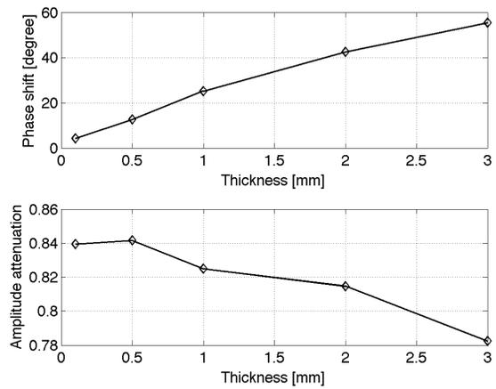
Figure 5: Dependence of phase shift (up plot) and amplitude attenuation (down plot) on the thickness of the beam pipe.
