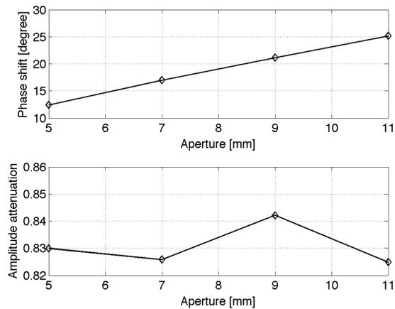
Figure 6: Dependence of phase shift (up plot) and amplitude attenuation (down plot) on the beam pipe aperture.
