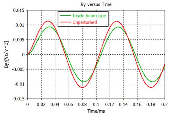
Figure 2: Magnetic field inside the beam pipe compared with the unperturbed signal.
