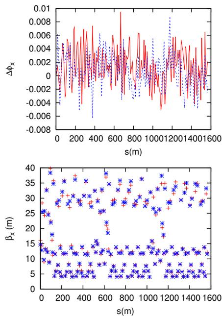
Figure 1: Measured horizontal betatron phase difference from a setting lattice and beta function evaluated by the phase.
