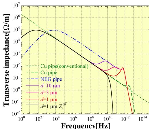
Figure 4: Transverse impedance per unit length of NEG-coated Cu pipes ( $d=1, 3$  and  $10 \mu\text{m}$ ) with  $b=12.5 \text{ mm}$  and effective impedance of the NEG-coated Cu pipe ( $d=1 \mu\text{m}$ ) shown by solid lines. The broken lines show transverse impedances for pure Cu and NEG pipes with  $b=12.5 \text{ mm}$  and the conventional expression for the pure Cu pipe.
