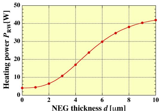
Figure 3: Heating power per unit length of the NEG-coated Cu pipe with  $b=12.5 \text{ mm}$  as a function of NEG thickness  $d$ .
