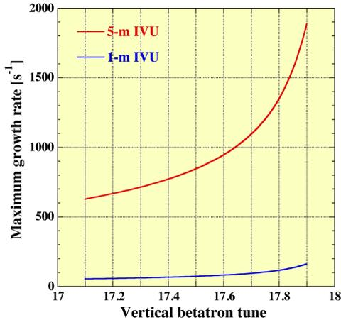
Figure 1: Maximum growth rate of the transverse instability due to a 5-m IVU in the long straight section and a 1-m IVU in the short straight section for the magnetic gap of 4 mm and the total current of 500 mA as a function of vertical betatron tune.
