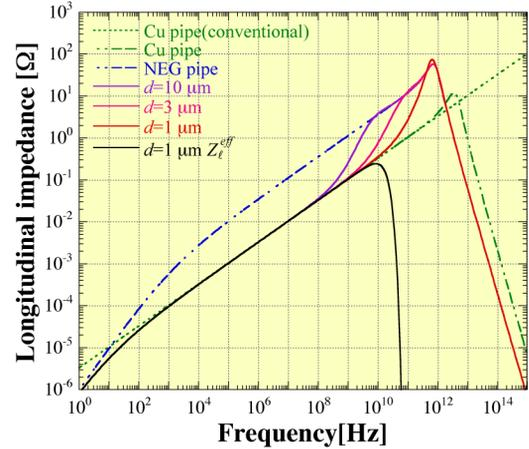
Figure 2: Longitudinal impedance per unit length of NEG-coated Cu pipes ( $d=1, 3$  and  $10 \mu\text{m}$ ) with  $b=12.5 \text{ mm}$  and effective impedance of the NEG-coated Cu pipe ( $d=1 \mu\text{m}$ ) shown by solid lines. The broken lines show longitudinal impedances for pure Cu and NEG pipes with  $b=12.5 \text{ mm}$  and the conventional expression of Eq. (1) for the pure Cu pipe.
