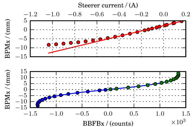
Figure 2: A steerer was used to deflect the beam giving an asymmetric measurement due to aperture (septum). Calibration of the BBFB was found by comparison of current normalized ADC counts (blue) and BPM values (red). Assuming symmetric behaviour the measured counts are extended (green). The interpolation (blue line) is further on used to calibrate current normalized BBFB counts to an offset in mm.
