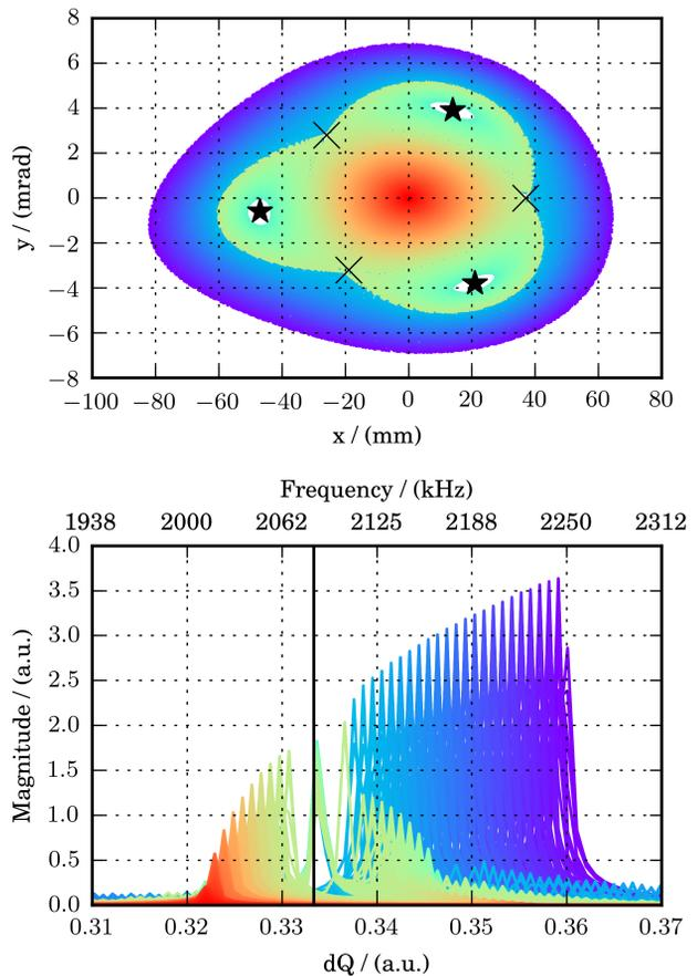
Figure 5: Tracking results for many particles starting at different offsets in  $x$  (colors) for the island optics of the MLS. The phase space plot nicely illustrates the core (red), island ( $\star$ ) and enclosing bucket (blue) as well as the unstable fix points ( $\times$ ). Below the corresponding frequencies are shown.
