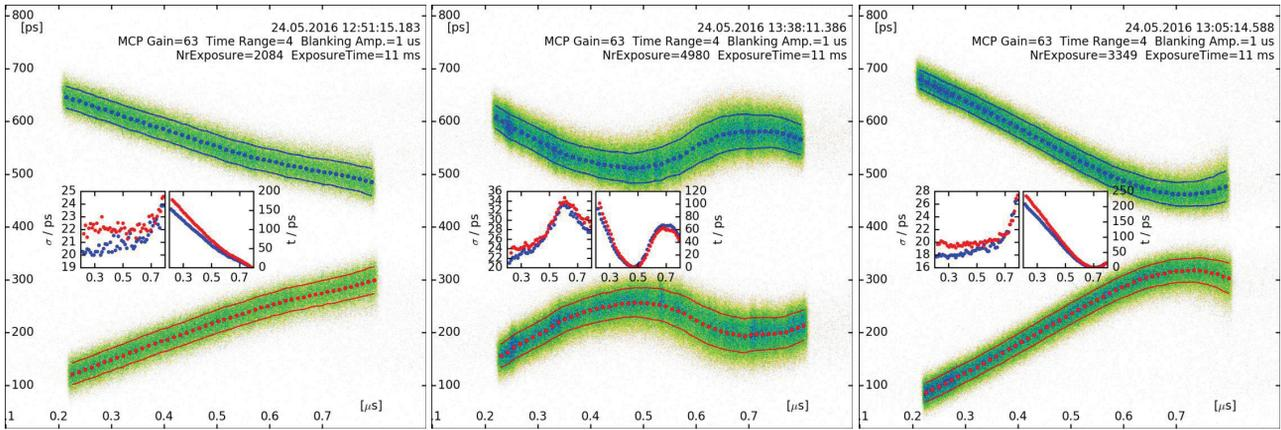
Figure 1: Streak camera images, photon counting, of high current operation with 100 ns gap in fill pattern. One main cavity in passive operation at  $h + 1$ , with the resonance frequency tuned to  $f \approx 400.5 f_{rev}$  (left),  $f \approx 401.04 f_{rev}$  (center) and  $f \approx 400.97 f_{rev}$  (right).
