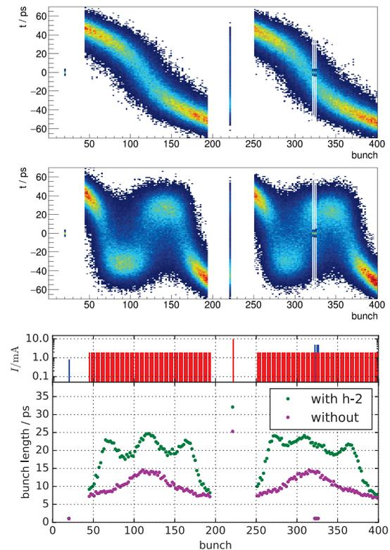
Figure 4: Simulation of phase transient and bunch length in BESSY VSR. Top: Without  $h-2$  cavity. Center: With  $h-2$  cavity. Bottom: Fill pattern and comparison of bunch lengths.
