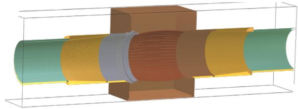
Figure 5: GdfidL model for the gate valve.
