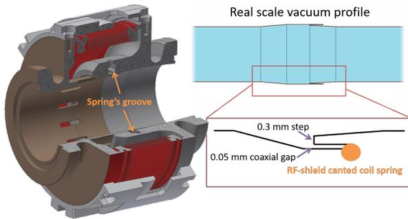
Figure 8: Telescopic bellows project and sketch.
