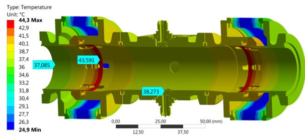
Figure 10: Case 2 thermal simulation for the BPM block.
