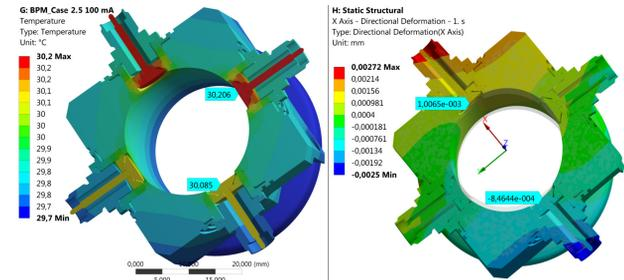
Figure 11: Thermal (left) and structural (right) analysis for the uneven worst-case load.
