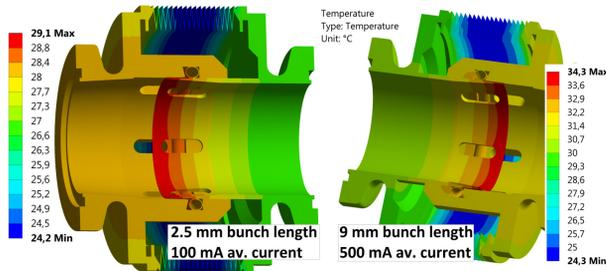
Figure 9: Thermal simulation for telescopic bellows: Case 1 (left) and Case 2 (right).
