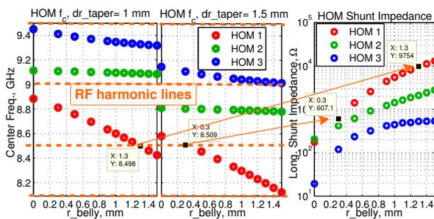
Figure 4: Valve HOMs shift and shunt impedance impact.
