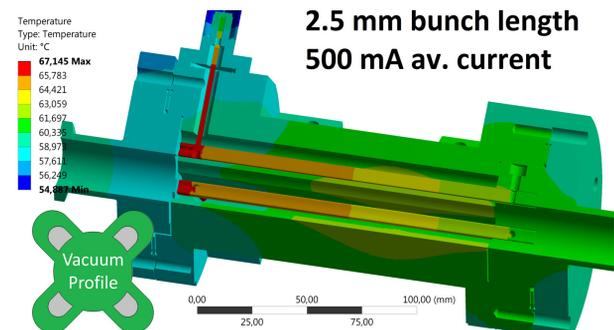
Figure 7: Thermal analysis of the stripline tune monitor.
