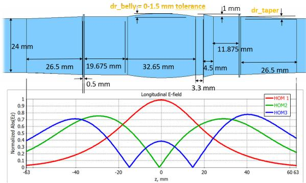
Figure 3: Longitudinal E-field distribution of the first 3 HOMs trapped in valve cavity profile.
