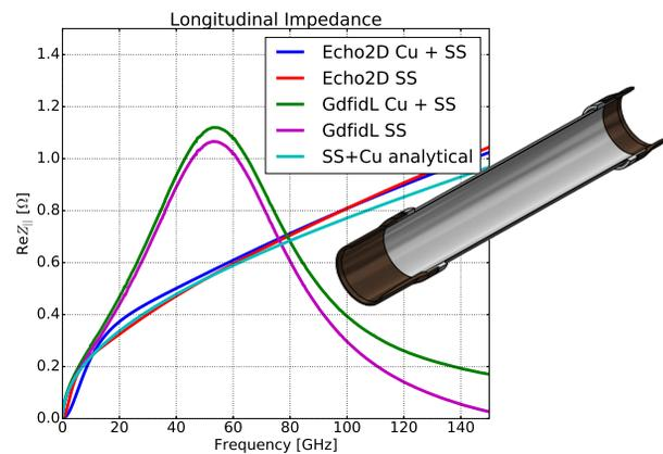
Figure 1: Real part of the longitudinal impedance of fast corrector chamber: comparison between ECHO2D, GdfidL – with and without copper pipe terminations – and theory.
