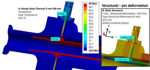
Figure 6: Analysis for the stripline kicker: thermal (left) and structural (floating right).
