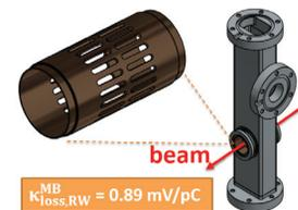
Figure 2: Mech. design for round chamber pump station.
