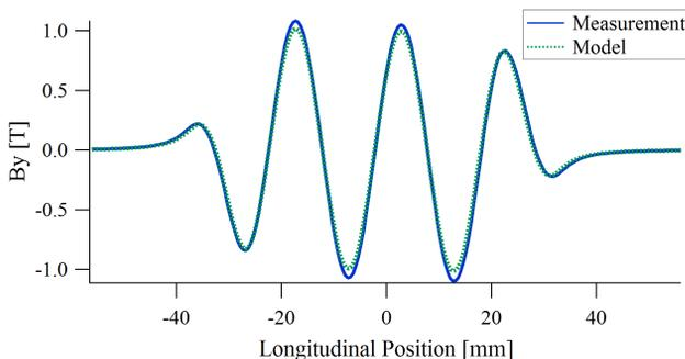
Figure 5: Vertical magnetic field component measured along the beam axis in the horizontal polarization phase. Dashed lines show the model calculation.
