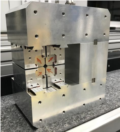
Figure 4: Prototype of the Sirius Delta-type undulator.
