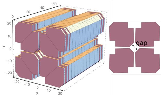
Figure 1: Magnetic blocks arrangement of the Sirius Delta-type undulator.
