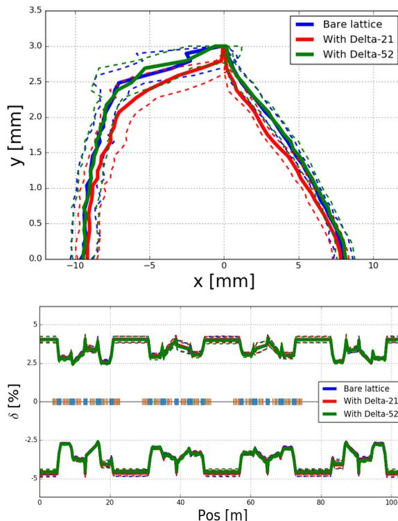
Figure 3: Dynamic aperture and momentum acceptance for the storage ring bare lattice (blue), lattice with 14 Delta-21 (red) and lattice with 14 Delta-52 (green). The dashed curves indicate one standard deviation from the average (solid curve) over 20 random machines.
