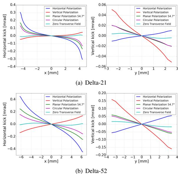
Figure 2: Total on-axis kick for the Delta-21 (top) and Delta-52 (bottom) IDs.
