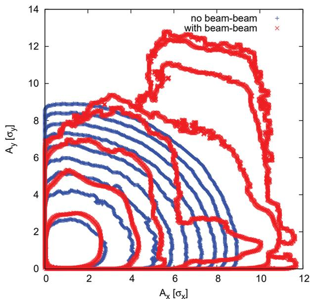
Figure 1: Transverse electron density distribution with (red) and without (blue) beam-beam interaction. The contour lines are spaced by a factor 10.
