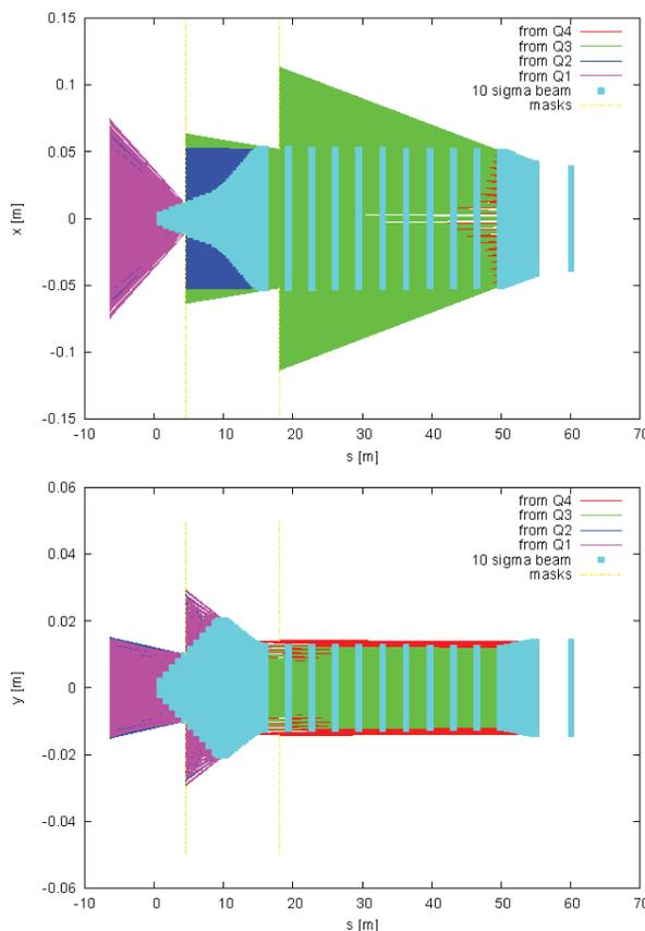
Figure 2: Synchrotron radiation fans from the last four quadrupoles through the IR, top view (top) and side view (bottom).
