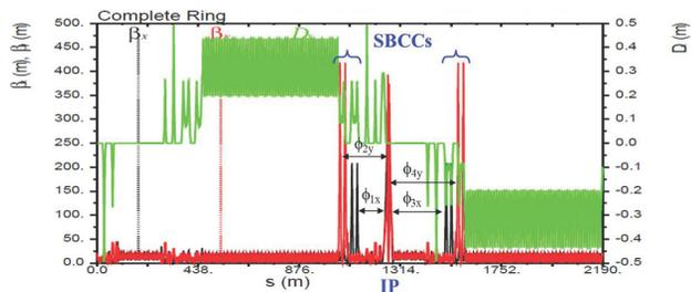
Figure 4: Electron ring optics with short-FODO arc cells and two SBCCs. Betatron tune is 57.22, 55.16 ( $x, y$ ).
