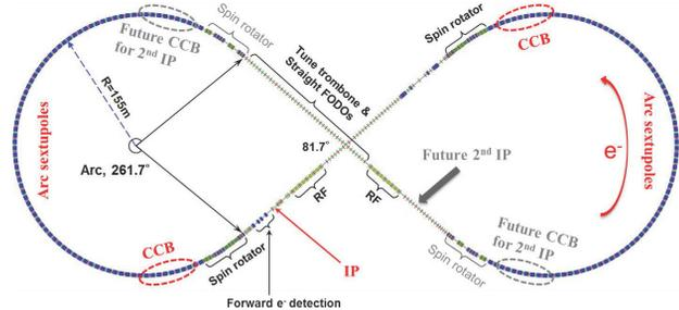
Figure 1: Layout of the 2.2-km electron collider ring.
