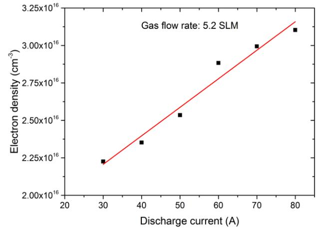
Figure 9: Electron density as a function of discharge current.
