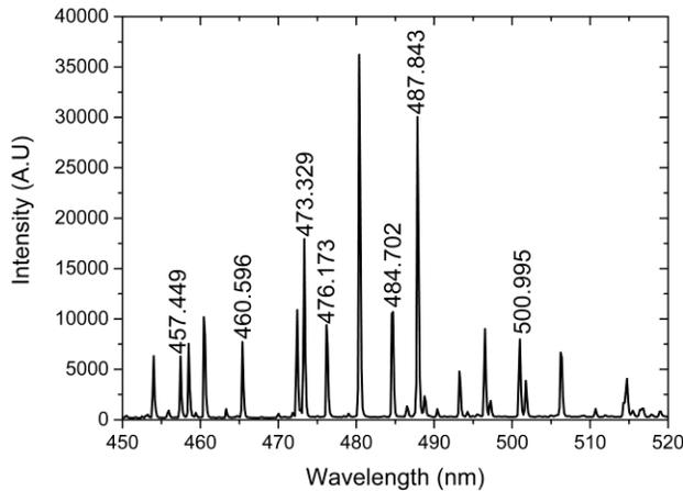
Figure 3: Emission spectra of Ar II lines in the spectral range of 450-520 nm.
