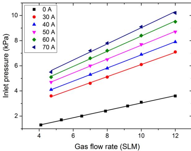
Figure 11: The inlet pressure of argon gas as a function of gas flow rate.
