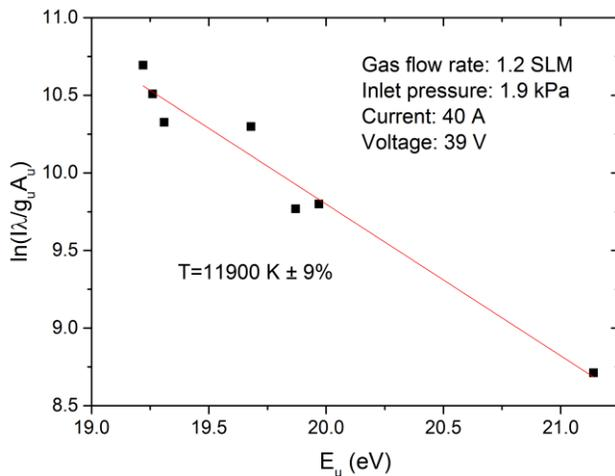
Figure 4: Typical Boltzmann plot for seven selected Ar II emission lines.
