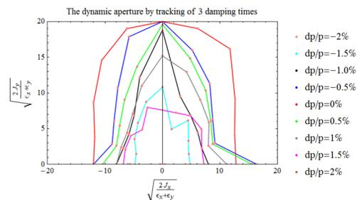
Figure 7: The dynamic aperture after reduce the synchrotron radiation energy per turn was reduced to one twentieth of the nominal.
