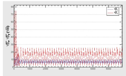
Figure 5: The sawtooth effect on the beta functions for 1/8th of the ring. The beta-beating is clearly shown. The  $\beta_y^*$  changed from 3 mm to 415 mm due to the strong energy sawtooth effect which comes from synchrotron radiation.
