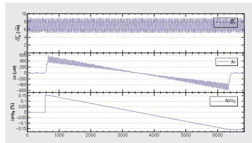
Figure 2: The beta function, closed orbit and energy saw tooth in one arc section of the ring. The maximum sawtooth orbit due to synchrotron radiation is  $\sim 6$  mm, while the maximum energy spread is  $\sim 0.15\%$ .
