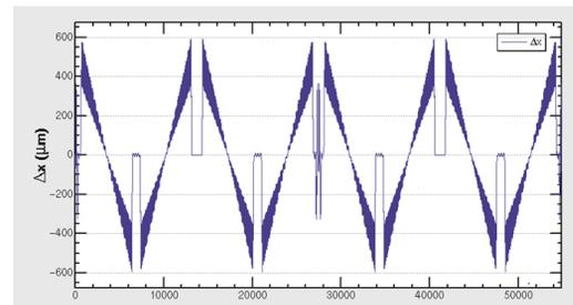
Figure 6: The saw tooth orbit along the ring due to the synchrotron radiation effect.
