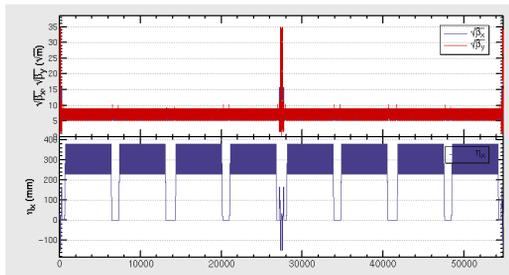
Figure 4: Beta functions and the dispersion function of the ring with final focus system before turn on the energy sawtooth effect.
