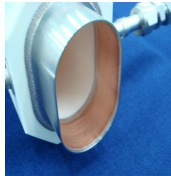
Figure 5: Cu conducting layer inner wall of Kovar sleeve.
