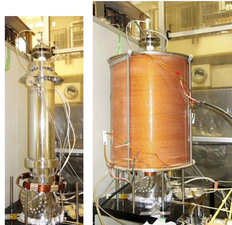
Figure 4: Sputtering machine for Ti coating.
