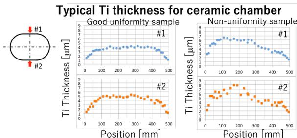
Figure 3: Ti coating thickness distribution inner wall of the ceramic along the beam longitudinal direction.
