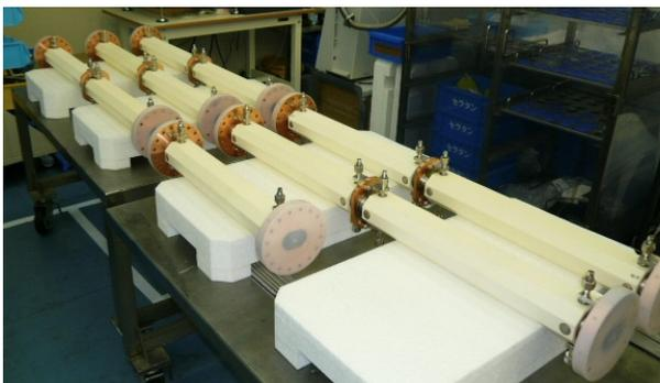
Figure 2: Ceramic chamber for abort kicker magnets.
