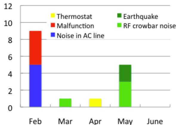
Figure 1: Monthly frequency of major failure occurrence is shown for the MW class power supplies.
