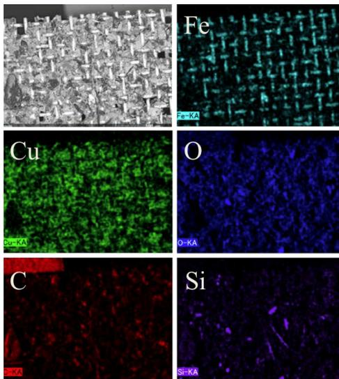
Figure 6: SEM analysis photos show that there are iron, copper, oxygen, carbon and silicon in the deposit. The pattern of the strainer mesh is clearly seen in upper left photo.
