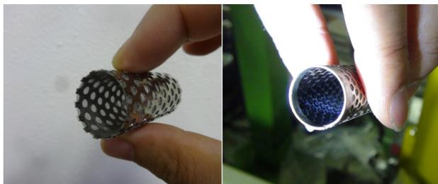
Figure 5: New strainer (left) and clogged strainer (right) are shown.
