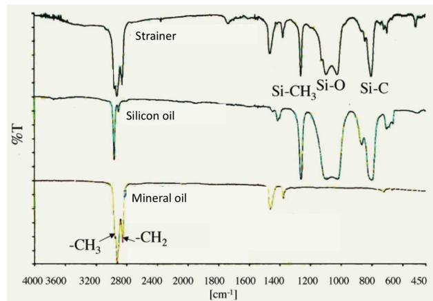
Figure 7: Infrared absorption spectra of the deposit sample of the strainer (top), Silicon oil (middle), and mineral oil (bottom) are shown.
