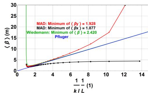
Figure 4: Deviation in both planes of optics from ideal FODO cell conditions in Pfluger and Wiedemann approximations. The vertical plane is broken by the delay chicanes, the horizontal plane by the radiator undulator focusing.
