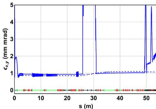
Figure 10: Normalised emittances along CLARA for Short 240 MeV/c mode.
