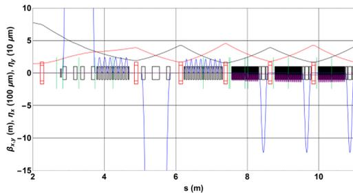
Figure 7: Optics (black/red) and dispersion (blue/purple) in both planes in chicane, modulator and radiator sections.
