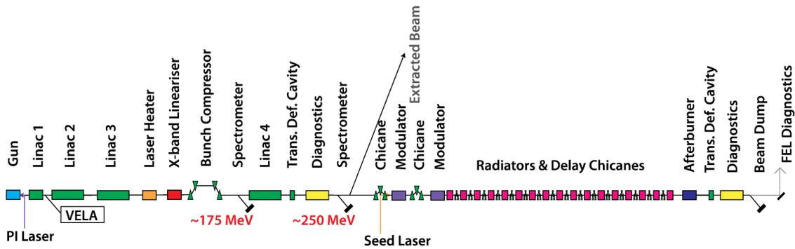
Figure 1: CLARA layout. The total length is ~ 90 m.
