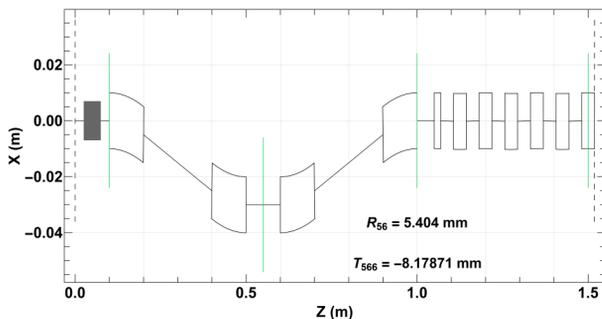
Figure 3: Seed laser chicane allowing for insertion of up to 100 μm seed.
