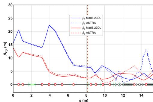
Figure 6: Optics matched from Linac-4 through TDC diagnostics section, seed laser chicane and modulators to radiator-1 in Mad and ASTRA.
