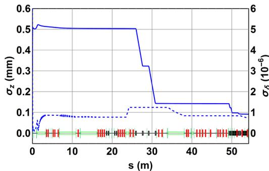
Figure 9: Bunch length and energy spread along CLARA for Short 240 MeV/c mode.
