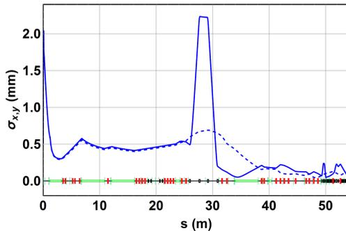
Figure 8: Matched beam sizes along CLARA for Short 240 MeV/c mode.
