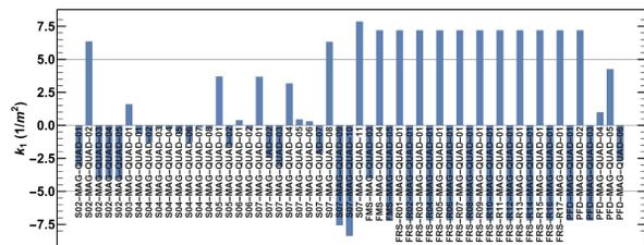
Figure 5: Quadrupole k-values from cathode through FEL to dump. Matched using ASTRA
