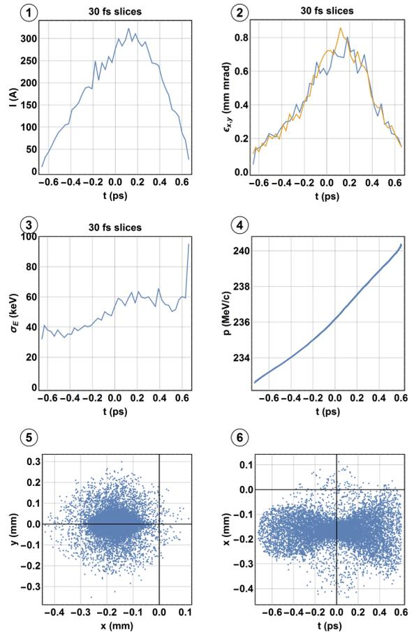
Figure 11: Tracked 10k bunch properties at FEL entrance, 30 fs slices where relevant. 1) Current profile. 2) Slice emittances. 3) Slice energy spread. 4) Longitudinal phase space. 5) Screen image. 6) x-t projection
