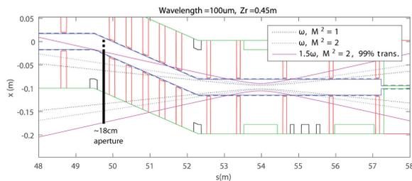
Figure 2: Aperture required by seed laser radiation mode in CLARA modulator-1 in rejected dogleg design.
