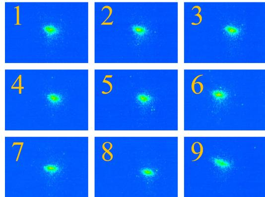
Figure 5: Turn-by-turn beam profile after PSM was on. The numbers correspond to the turn number after the PSM on.
