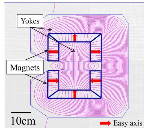
Figure 2: Cross section of permanent bending magnet design.
