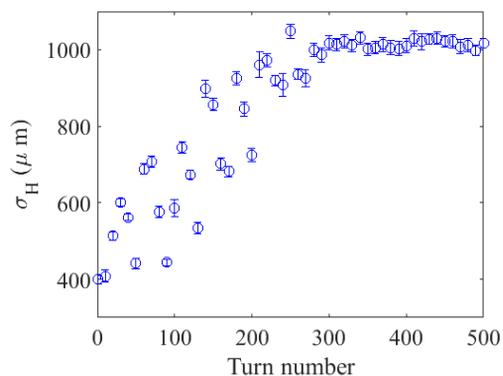
Figure 6: Change in horizontal beam size after PSM kick
