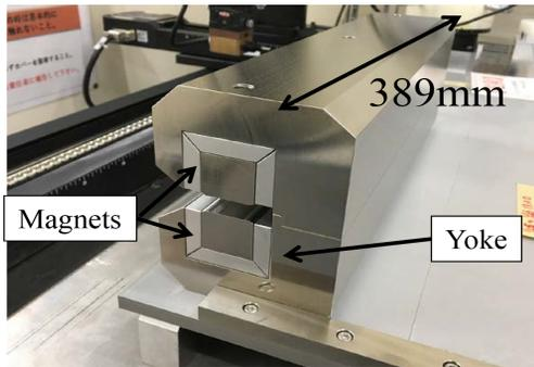
Figure 3: Photograph of 1/5 model magnet.
