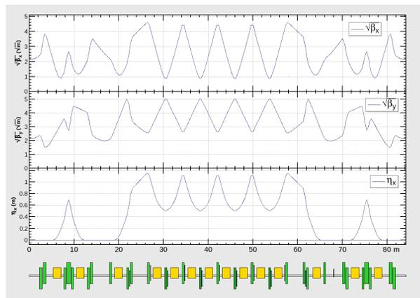
Figure 2: Optical functions of the booster ring. The booster ring is the dyad-symmetrical.
