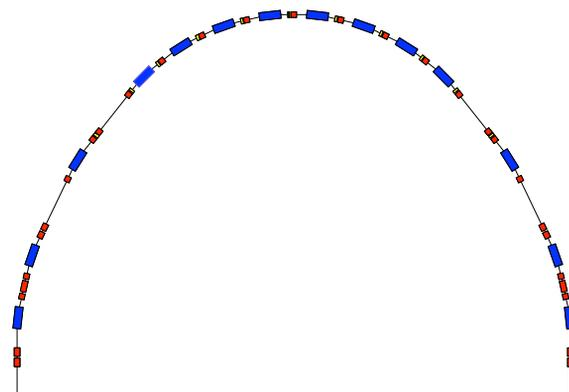
Figure 3: Lattice of the half of the booster ring. Blue boxes show the bending magnets, red the quadrupole magnets and yellow the sextupole magnets.
