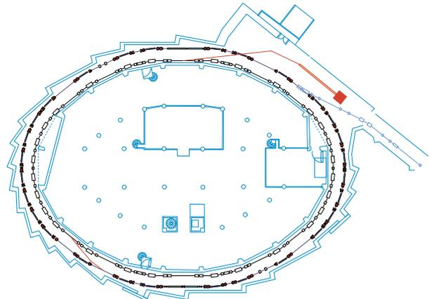
Figure 1: Configuration of the new injector system. The small linac consists of an electron gun (red square) and one accelerating structure (bold orange line). The orange line shows the schematics of the beam transport line.
