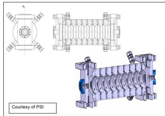
Figure 4: Design of the RF structure short prototype.
