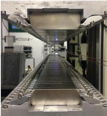
Figure 5: New modulator magnetic array.
