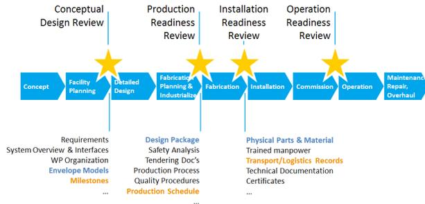
Figure 5: Project lifecycle with engineering reviews and examples for their content. Colors indicate the evolution of engineering design and schedule.
