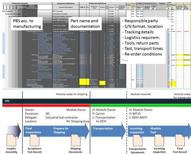
Figure 3: Sample MBOM (top) and excerpt from fabrication and test process (bottom).
