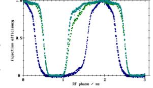
Figure 3: Accumulation efficiency as a function of the RF-phase with off-axis injection and non-optimized (blue) and after first and second optimization of sextupole settings (green and light blue).
