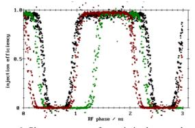
Figure 6: Phase acceptance for optimized sextupole settings and total accelerating voltages of 600, 1170 and 2100 kV (red, black and green).
