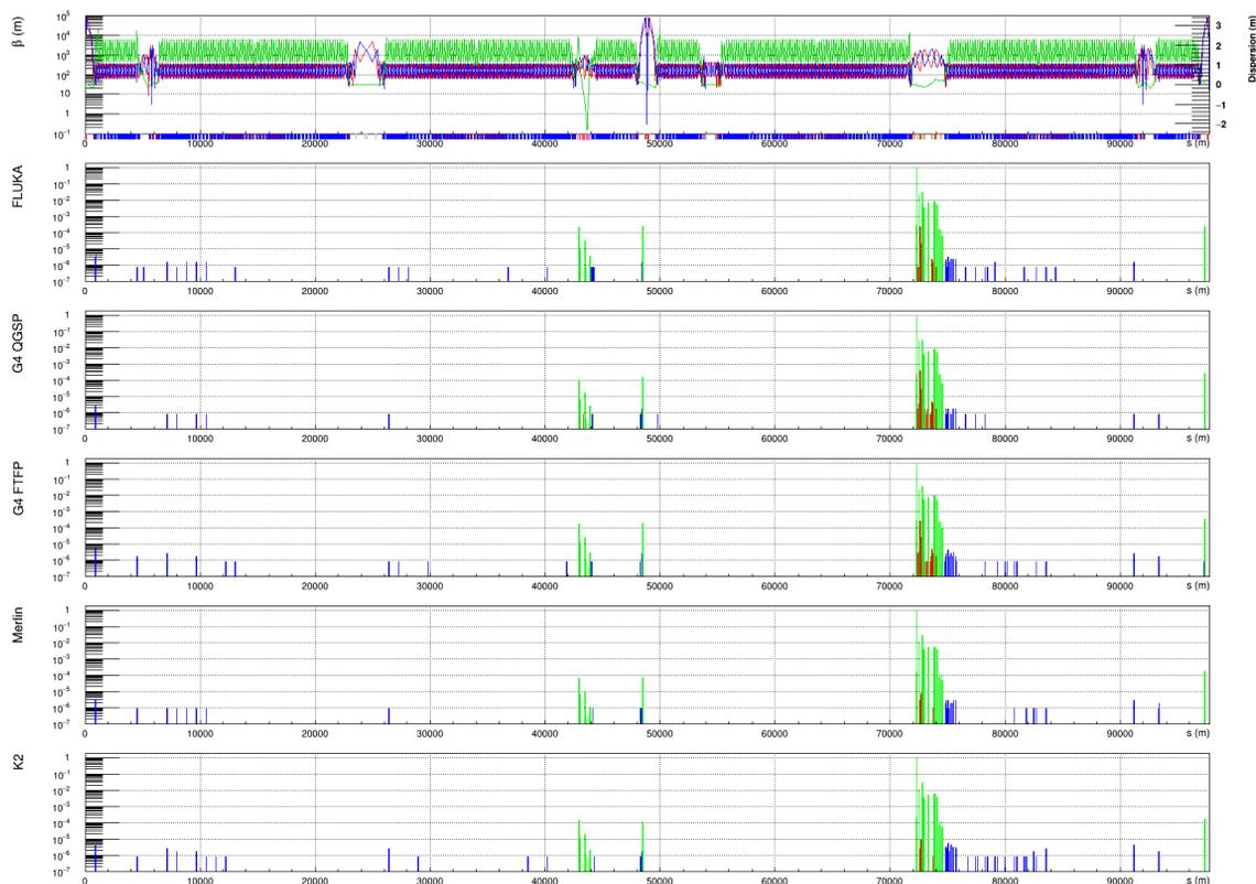
Figure 2: An image showing loss maps using each code for the FCC-hh collimation system, showing the full accelerator ring. Green losses are at collimators, red are warm magnets, and blue are at cold superconducting magnets. The upper plot shows the lattice optics, with the transverse beta functions being in red and blue, and the horizontal dispersion function shown in green. Further information is given in [22, 23].
