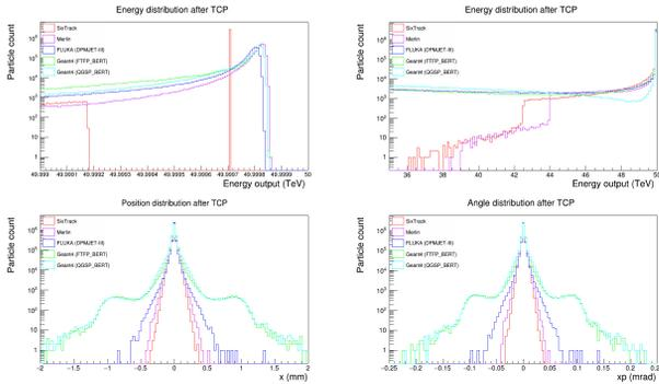
Figure 1: Histograms showing the outgoing phase space distributions from 50 TeV protons impacting a single test collimator jaw.
