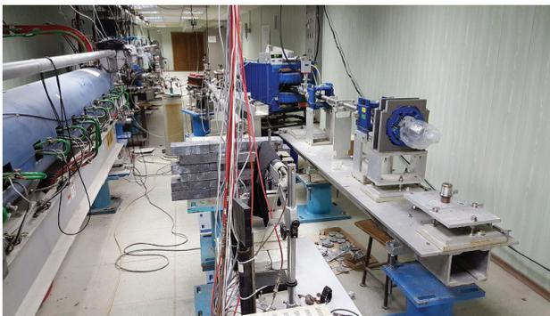
Figure 4: Current setup of the 22 MeV part of Linac-200. From left to right: main accelerator beamline, user beamline, training beamline.
