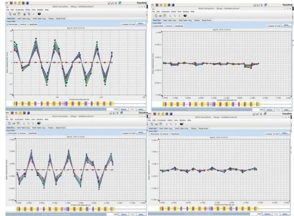
Figure 2: The COD correction performed in RCS. The left two diagrams represent the COD before correction in horizontal and vertical respectively, and the right two diagrams represent the COD after correction in horizontal and vertical respectively.
