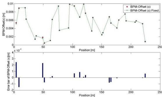
Figure 1: Top: the comparison of horizontal BPM offset between simulated and fixed respectively; Bottom: the error bar of horizontal BPM offset.
