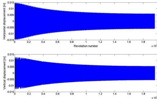
Figure 3: The simulated bunch by bunch data of one BPM. The upper and bottom represent horizontal and vertical respectively.
