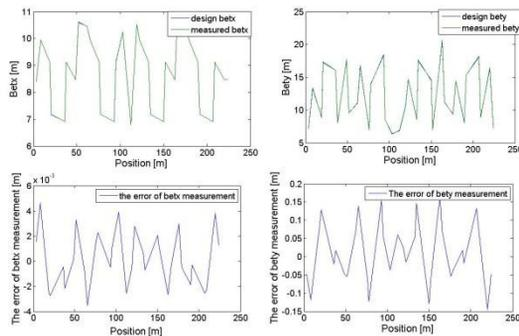
Figure 4: Beta functions decomposed by SOBI. Two graphs at the top represent the horizontal and vertical beta function respectively; and two graphs at the bottom represent the beta-beating in horizontal and vertical respectively.
