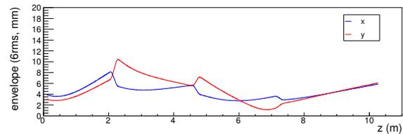
Figure 8: Beam envelope of the DLS section.
