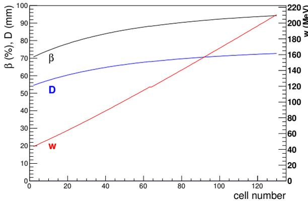
Figure 2: Calculated cell parameters of the DLS section.
