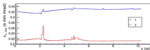
Figure 7: Emittance evolution through the DLS section.
