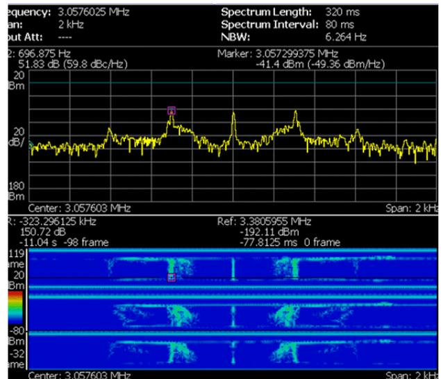
Figure 2: the spectrum image of 290 MeV/u beam ( $V_{rf} = 280V$ ).
