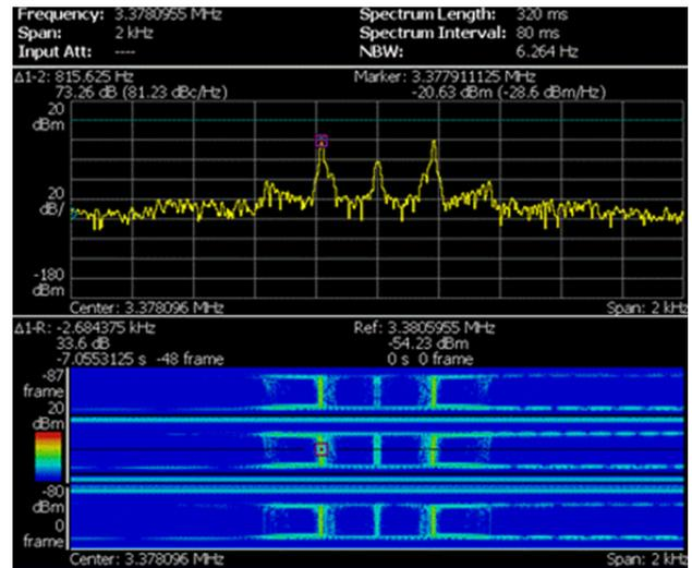
Figure 1: the spectrum image of 400 MeV/u beam ( $V_{rf} = 174V$ ).
