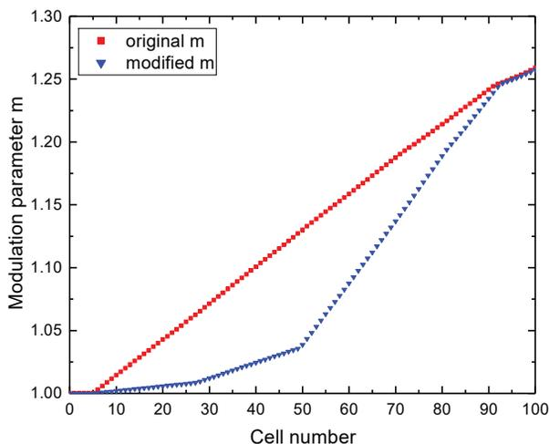
Figure 3: Plots of the modulation parameter  $m$  against the cell number for two cases: the red graph shows the original  $m$ -shape as produced by RFQGen, whereas the blue graph shows the modified  $m$ -shape.
