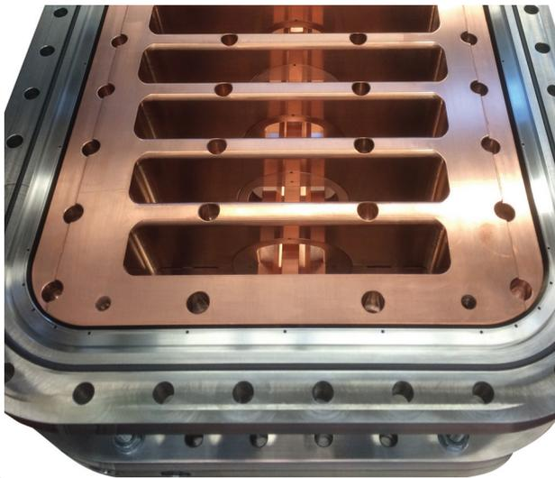
Figure 1: Photo of the Ladder-RFQ prototype (courtesy of M. Schütt). The upper steel-tank was removed to get a view of the inner ring-ladder structure.
