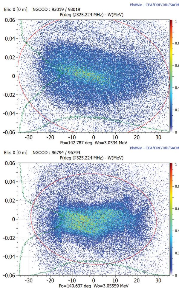
Figure 4: Plots of the longitudinal phase space distribution projections (green curves) at the RFQ exit in case of the original (top) and the modified (bottom)  $m$ -shape. The colors of the scatter plots refer to the normalized (macro) particle density (cf. scales at the right frames of the plots). The red ellipses refer to the normalized 90 % emittances.
