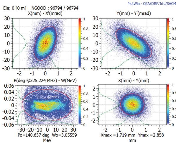
Figure 5: Phase-Space plots and distribution projections (green curves) at the RFQ exit in case of the modified  $m$ -shape. The colors of the scatter plots refer to the normalized (macro) particle density (cf. scales at the right frames of the plots). The red ellipses are associated to the normalized 90% emittances.
