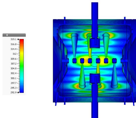
Figure 6: Result of a thermal simulation with the new cooling system inside MYRRHA CH-cavity number 5.
