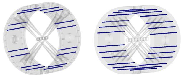
Figure 4: Comparison of the cooling channels inside the tank of the CH prototype (left side) and the MYRRHA CH-cavities number 1 to 7 (right side).
