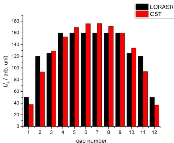
Figure 7: Comparison of the effective voltages of the CST and the LORASR simulation during the adjustment process.
