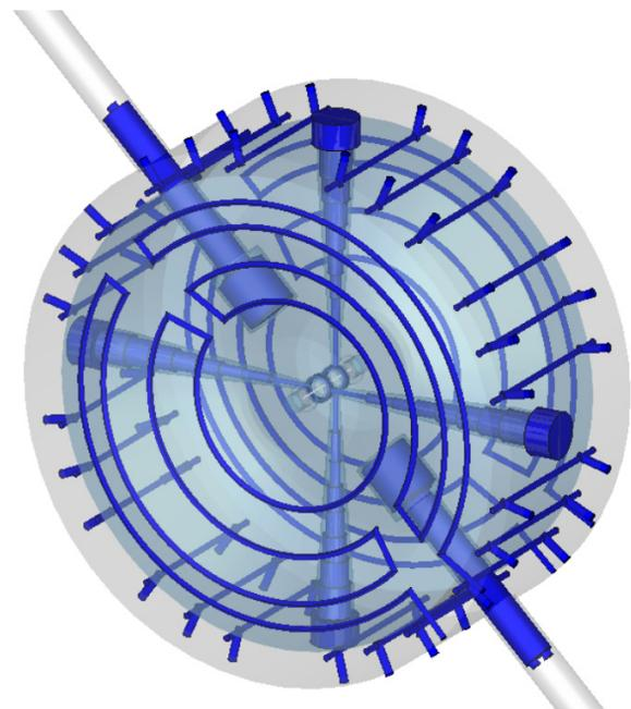
Figure 5: The complete cooling system of a MYRRHA CH-cavity.
