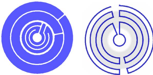
Figure 3: Comparison of the cooling channels inside the lids of the CH prototype (left side) and the MYRRHA CH cavities number 1 to 7 (right side).
