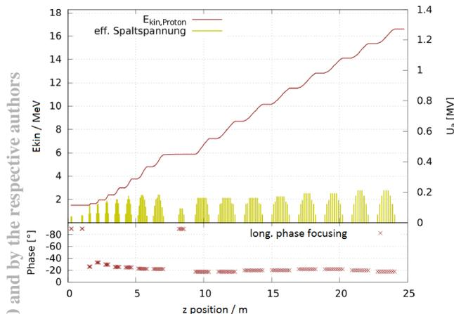
Figure 1: The estimated proton energy after the 4-Rod-RFQ is 1.5 MeV [5] and increases up to 16.6 MeV at the end of C H 15 (upper graph in red). The effective voltages of the gaps are plotted in yellow. The lower graph shows the constant phase configuration of the 15 cavities.
