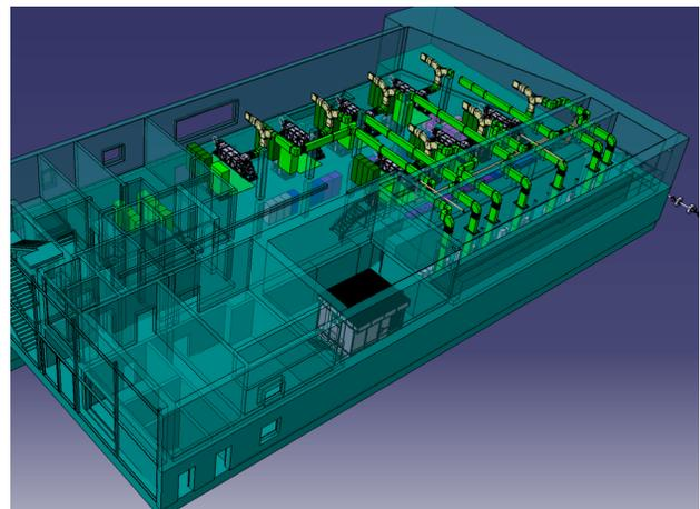
Figure 1: 3D view of the pLinac building including the RF support structures and the accelerator tunnel.
