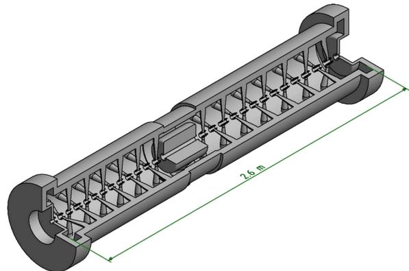
Figure 5: Final RF design of the 2nd coupled cavity CCH2.
