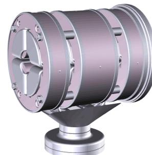
Figure 6: Magnetic triplet. RF housing only partly shown.
