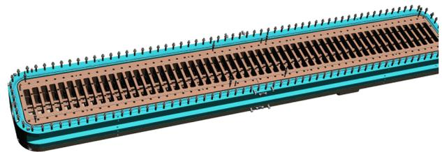
Figure 4: 3D model of the ladder RFQ illustrating the ladder structure with electrodes.
