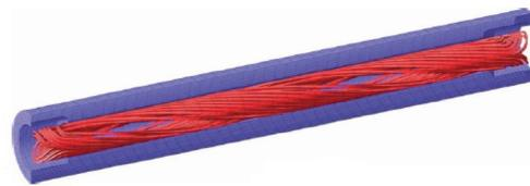
Figure 2: OPERA view of one 2.4 m,  $360^\circ$ -twist helix module of the 10.5 m long, 4-module RHIC snake.
